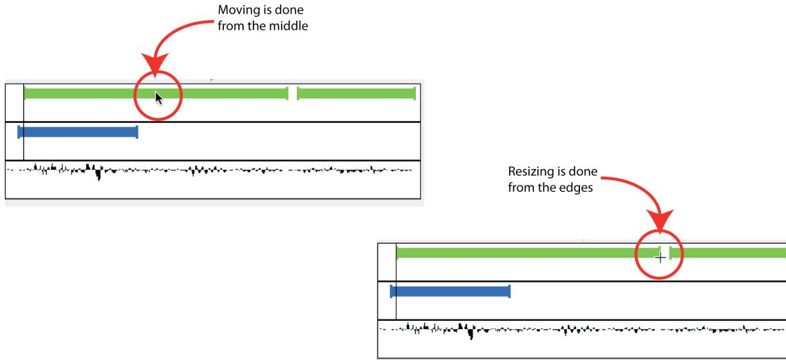
**Figure 3-3. Moving vs. Resizing Annotations.**
