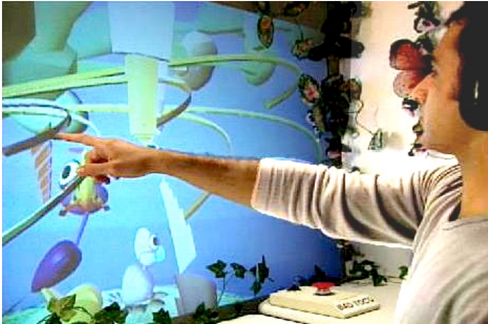
Figure 6-2: A player sits in front of a large screen which shows animated graphics. Overhead cameras are used to track the persons hands, and a head-worn microphone senses the player’s speech.
