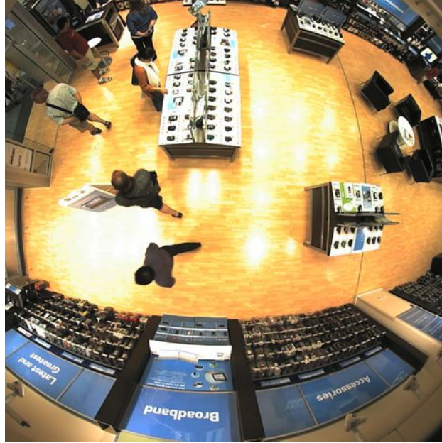
Figure 1.3: A typical frame of video from an in-store overhead camera. This frame is from the Best Buy Mobile case study described in Chapter 4. Video was recorded at 960 by 960 resolution at approximately fourteen frames per second.
