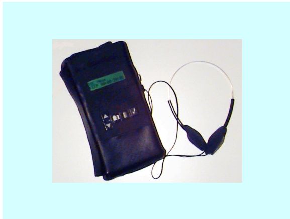
Figure 8 The NewsComm hand-held audio playback device with headphones
