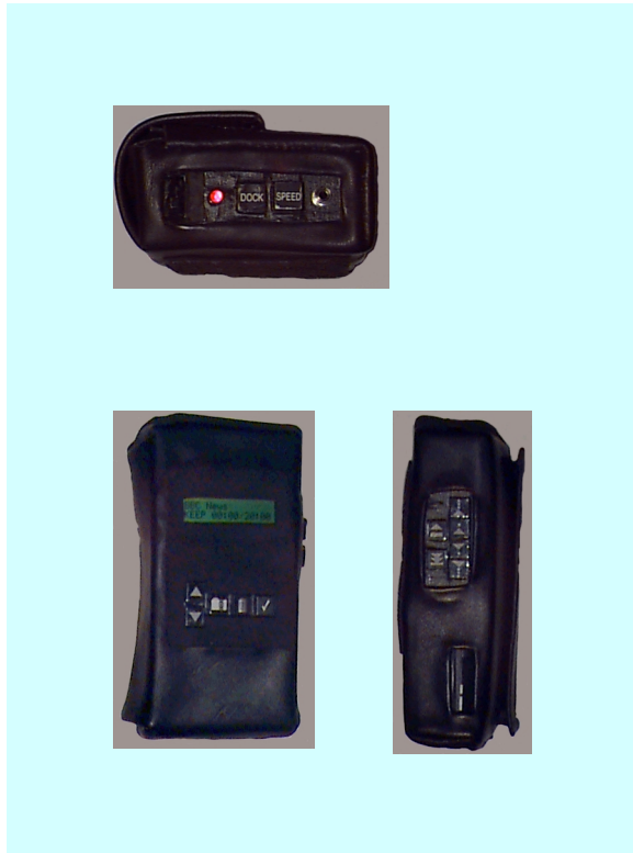
Figure 12 Details of the top, front, and right sides of the final hand-case, which incorporates Version 5 of the interface design
