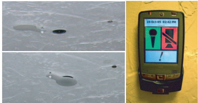
Figure 2: Top left: Camera and microphone embedded in ceiling with camera shutter open (the microphone is the small dark disk to the right). Bottom left: shutter closed. Right: Wall mounted touch display for recording control (see section on privacy management for details).
