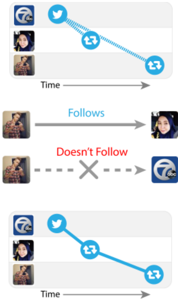
Figure 4-8: Using Twitter's follower graph to infer the correct retweet path of a tweet. The top panel shows the retweet path provided by the Twitter's API. The middle panel shows that the bottom user is a follower of the middle user but not that of the top user (the user who tweeted the original tweet). The third panel shows that using this information, and the fact that the bottom user retweeted after the middle user, we can infer that the bottom person retweeted the middle person and not the top person.
