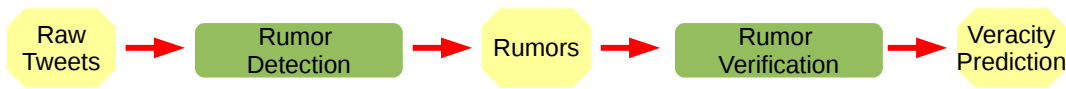
Figure 1-1: The pipeline of the rumor detection and verification system. The inputs and outputs are shown in yellow and the detection and verification subsystems in green. The rumor detection subsystem is named Hearsift and the the rumor verification subsystem is named Rumor Gauge .
