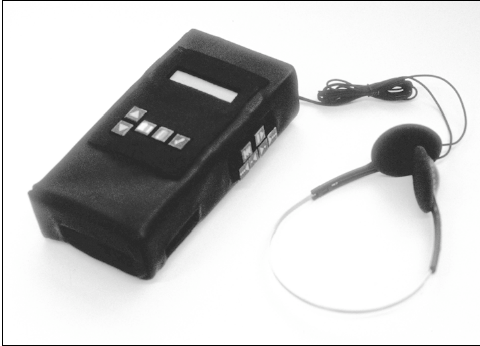
Figure 1: The NewsComm hand-held audio playback device with headphones. The top face houses a display and controls for selecting and managing recordings which have been downloaded into the hand-held's memory. The right side houses the navigation interface which can be controlled with the thumb while holding the device. The device can be connected to a central server to download personally selected digital audio recordings.
