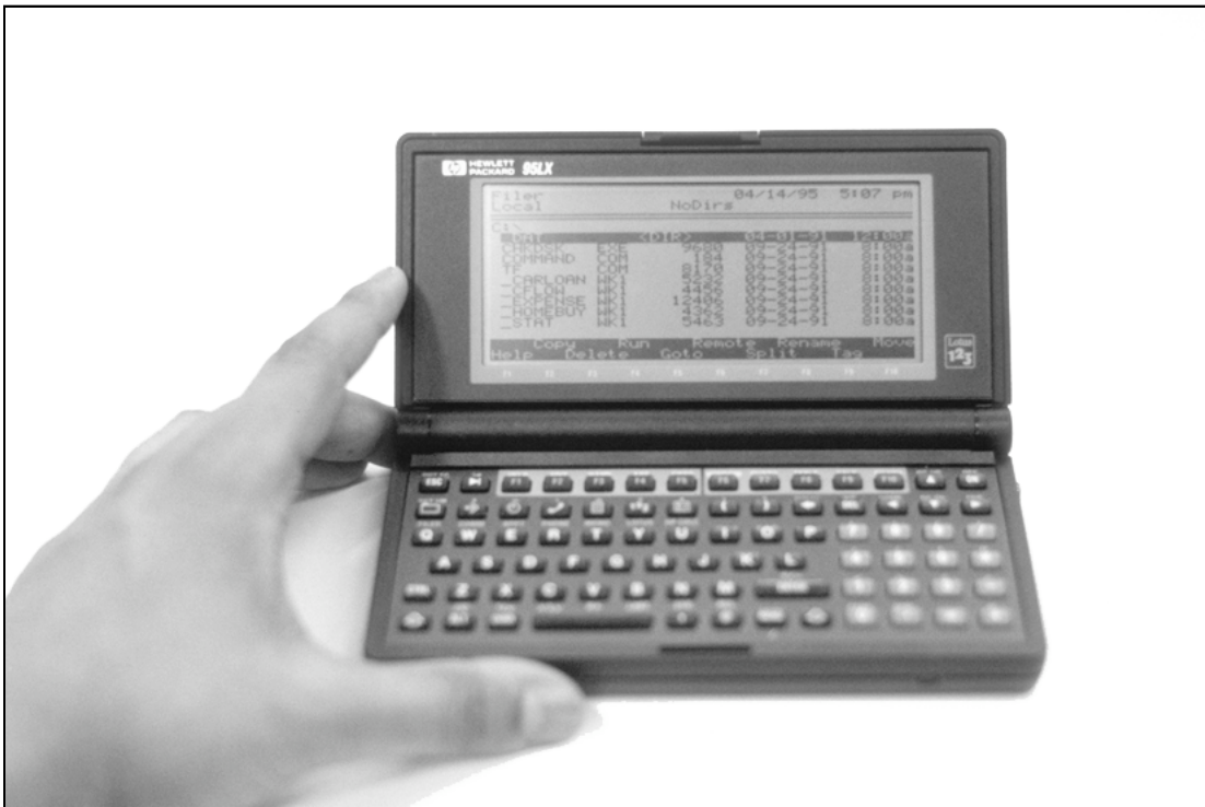
Figure 11: The HP95LX is an 11 ounce palmtop computer. It has a PC-XT architecture, contains a 80C88 compatible CPU, 512K of system RAM, an 8 bit digital-to-analog converter, a type II/III PCMCIA port, and a RS-232 serial port.
