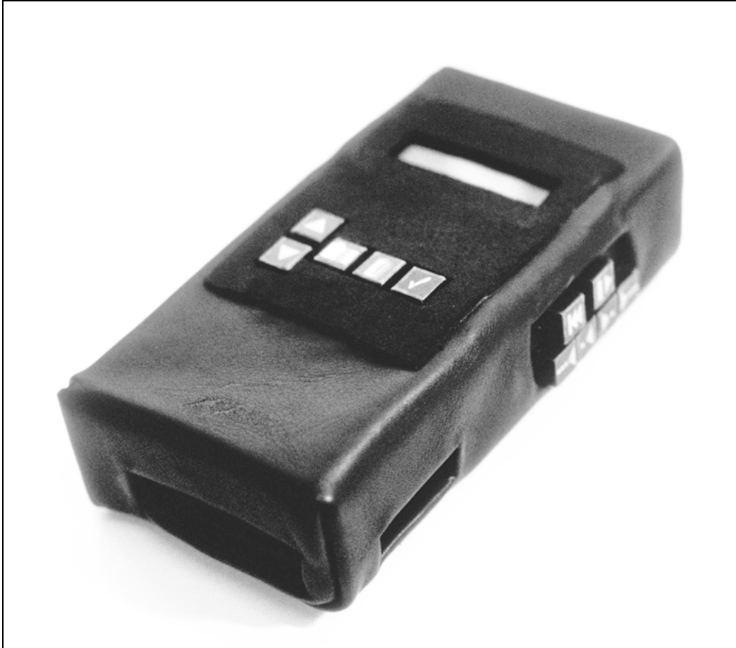
Figure 14: Photo of the final (version 3) hand-held. The case is made of soft black leather lined with cardboard supports from the inside. The HP95 is inside the case. The buttons are low profile tactile keyboard buttons. The screen is a 2 line by 16 character LCD module. The top panel (not in view) houses the main power switch, power indicator LED, headphone jack, and two buttons (the DOCK and SPEED buttons).
