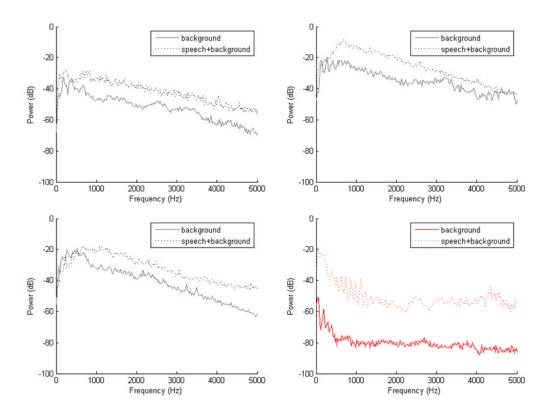
**Figure 7-2.** Sample power distributions showing effect of background noise in baseball video. Four audio samples compare the distribution of power during just background noise to the distribution of power during background noise plus speech. Top samples and lower left sample extracted from baseball video (in gray). Lower right sample generated under laboratory conditions (in red).
