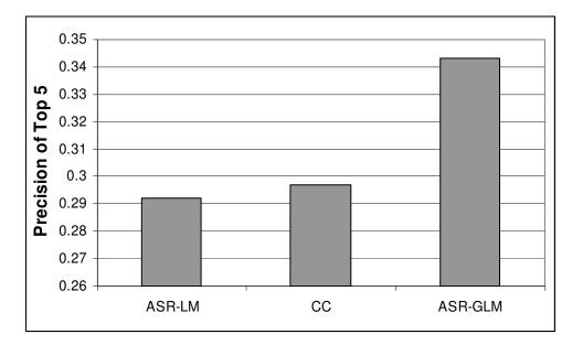
**Figure 7-4.** Precision of top five results of a video IR system based on speech transcriptions. Three different transcriptions are compared: ASR-LM uses ASR with a text-only interpolated language model (trained on baseball closed captioning and the switchboard corpus); ASR-GLM uses ASR with a grounded language model; CC uses human generated closed captioning transcriptions (i.e., no ASR).
