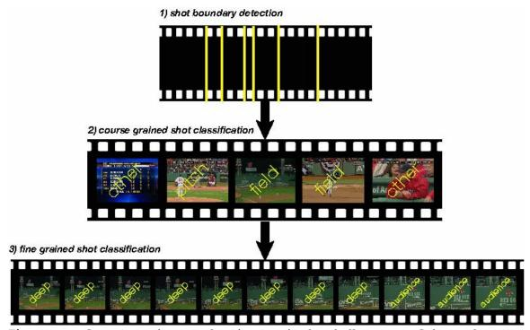
**Figure 5-2** Overview of scene classification for baseball games. Color and motion features are used to break raw video into individual shots. Key frames within each shot are then classified into course categories (i.e., field, pitch, other). Shots categorized as *field* are then broken into sub key frames (one for every ten frames) and sub-categorized.
