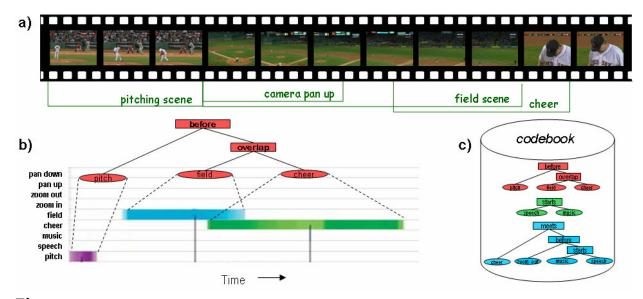
**Figure 5-1.** Overview of Event Representation in Video. a) Events are represented by first abstracting the raw video into visual context, camera motion, and audio context features. b) Temporal data mining is then used to discover hierarchical temporal patterns in the parallel streams of features. c) Temporal patterns found significant in each iteration are stored in a codebook that is used to represent high level events in video.
