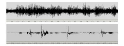
**Figure 7-1.** Sample waveforms showing the effect of magnitude of background noise in baseball audio noise. Both waveforms are of the same utterance: "into left center field for a base hit." The bottom utterance was spoken in controlled laboratory conditions. The top utterance was taken from the audio stream of a broadcast baseball game.
