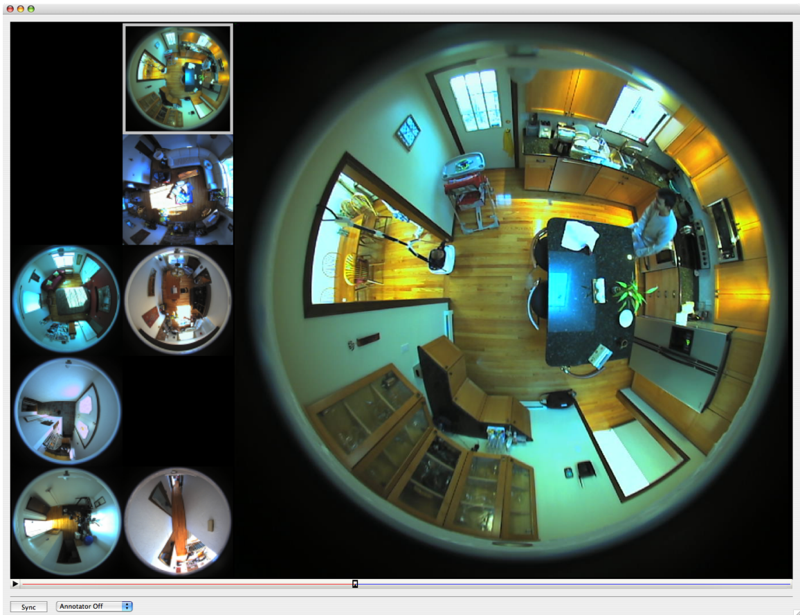
Figure 2-8: TotalRecall video player. On the left are low resolution videos from all cameras that are currently on. On the right is a full resolution (about 1000x1000 pixels) video from the kitchen, which is the currently selected channel.
